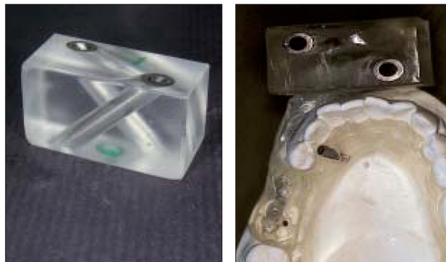
Fig 1a (Left) An acrylic resin cube, which includes 2 precisely positioned tubes made of titanium, is used to make a link between the planning software and the drilling machine.
